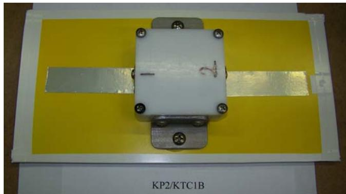
Figure 4. Painted panel with mounted CHM and tape electrodes.
