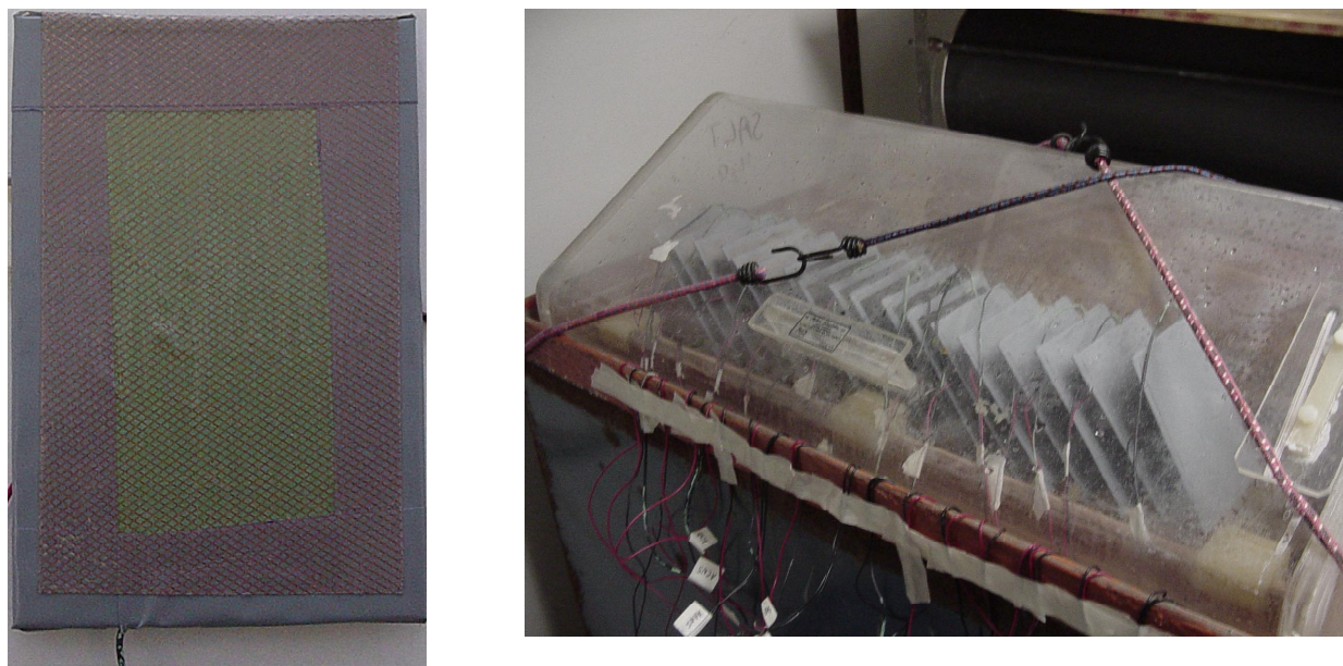
Figure 5. Left) Representative specimen with clear appliqué showing sensor electrode underneath. Right) Specimens in salt fog.
