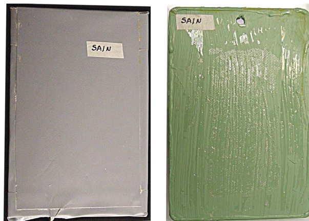
Figure 6. Example of no-defect steel specimens before and after appliqué removal.
